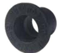
16MM GROMMET (19MM HOLE RQD) PF919/16
